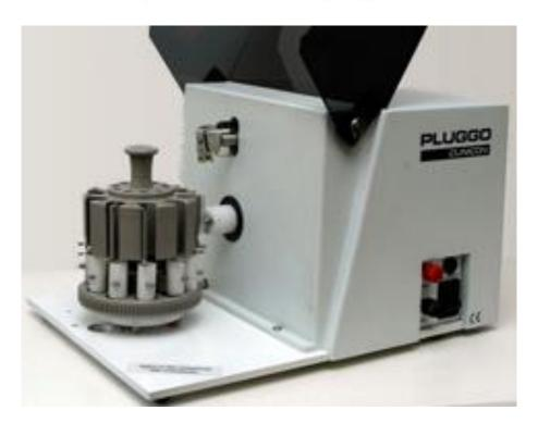
The caps are guided to an outlet for collection of biohazard disposal with a detachable chute.
