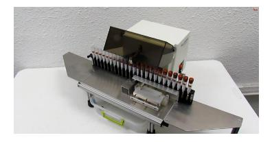
A detachable chute guides the caps into a disposal area beneath the instrument after decapping.
